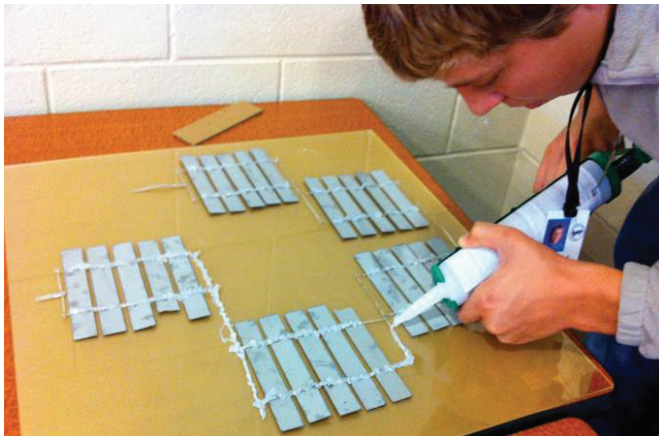
Student prepares a protective layer of cushioning for fragile silicon cells that are used as part of a student-created Solar Photovoltaic Panel.
