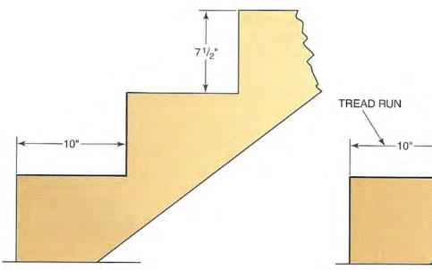
17-18 METHOD – ONE RISE PLUS ONE TREAD RUN SHOULD EQUAL BETWEEN 17 AND 18 INCHES. TREAD RUN
