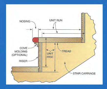
Two formulas are used to determine the unit run for stairs (Fig. 16-7).
